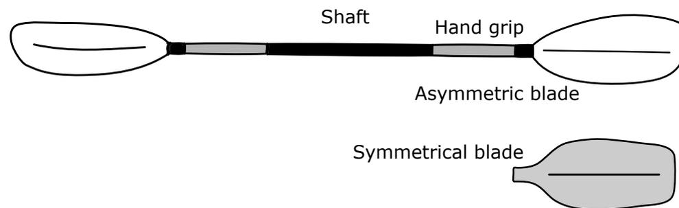
Blade shapes may vary, but the asymmetric shape, which reduces twisting, is now common in kayak paddles. Blade sizes also vary, and the temptation may be to use large blades thinking that they will give more power. However, bigger blades, especially on longer shafts, can lead to joint injuries. It's best to take advice before spending too much.
