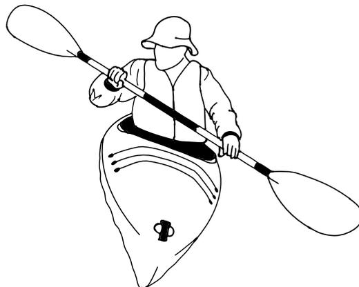
Kayak on edge: stable because centre of gravity is above centre of buoyancy
